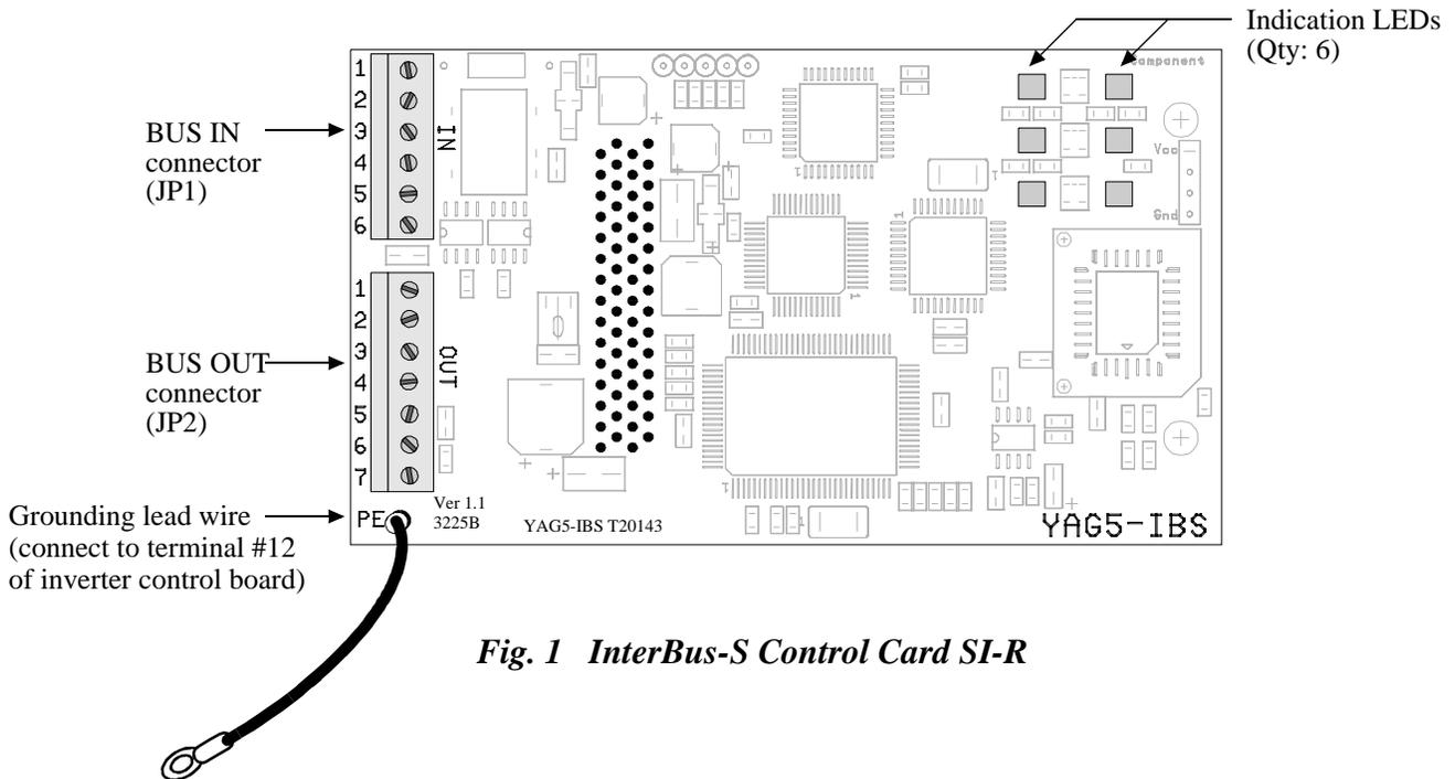
**Fig. 1 InterBus-S Control Card SI-R**
