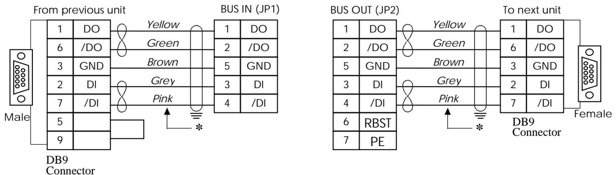
**Fig. 4 Wiring of the InterBus-S Control Card SI-R**
