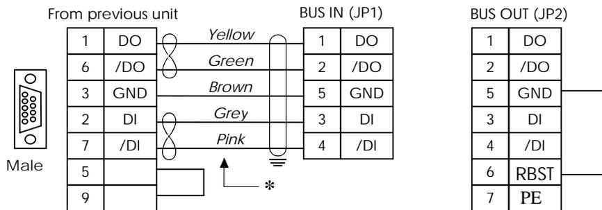
**Fig. 5 Installation of the RBST signal**
